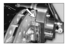
will seriously affect your brake performance. Should you encounter difficulty fitting the shims then remove the four pad return bolt/springs, fit the shim and refit the return bolt/springs.
