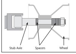
For setting the front track width, a good starting point is.
