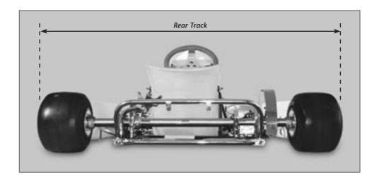
**Important:** Rear track is probably the most important single variable in a kart chassis. Different driving styles and different tracks will require different settings. The standard setting is the best starting point and we suggest you vary the rear track by no more than 5mm each side per change.
