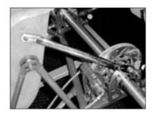
**Note:** Additional seat stays are available which fix to the axle bearing flanges and the top section of the seat. Testing has shown these to be advantageous under certain conditions and a disadvantage under others.
